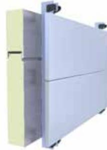
To accommodate thermal movement, the modular click rail SE is supplied pre-punched with alternative round and slotted holes. One fixed point is required per rail. The optimal configuration is to make the fixed point in the same position in each rail.
