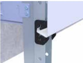
4. Install a fixed point clamp and guidance snapper(s) in the lower panel (see section 6.4) before hooking the second panel in place above.
