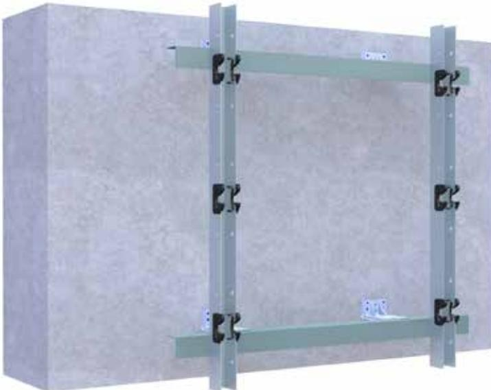
The modular click rail SE should be fixed to the horizontal cladding rails with the appropriate number of self drilling/tapping screws or rivets, taking account of thermal movement.
