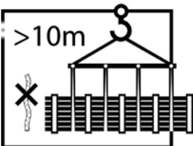
To reduce the risk of damaging FC panels, ropes should not be used. Slings with a minimum 150 mm width are recommended.
