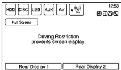
3. Press Rear Display 1 for the second row video screen and Rear Display 2 for the third row video screen (if equipped).
