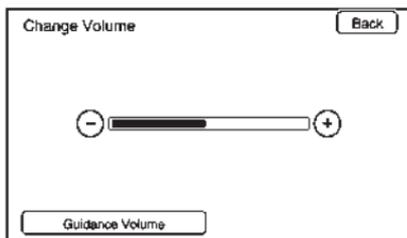
**Voice Volume:** Adjust the voice volume for guidance and voice recognition prompts by pressing – or + or by turning the Multifunction knob. Press the Guidance Volume screen button to preview the selected sound level.
