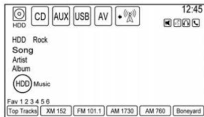
Press SRCE, cycle through the available audio sources until HDD displays, then press the HDD source button. You can also touch the audio page to toggle to HDD, then press the HDD source button.
