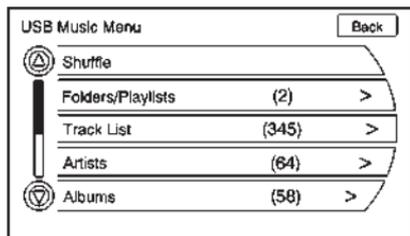
Press the USB Menu screen button or press the Multifunction knob while on the USB audio screen to display the USB Music Menu.
