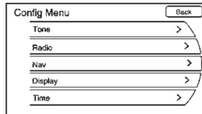
To access the Radio settings menu, press MENU to display the Config Menu. Turn the Multifunction knob to scroll through the available features until the Radio feature displays. Press this feature to display more options.
