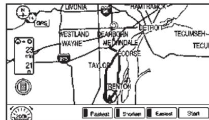
The POI destination entry allows selection of a destination by providing the POI name or a city name, by selecting from the POI list.
