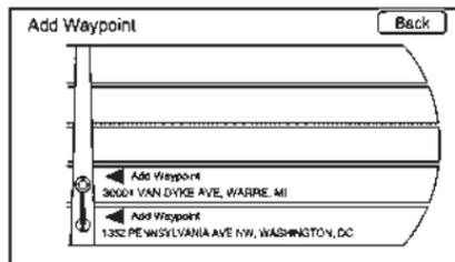
Up to three waypoints can be added to the current route, between the start point and final destination. The waypoints can be edited or deleted.
