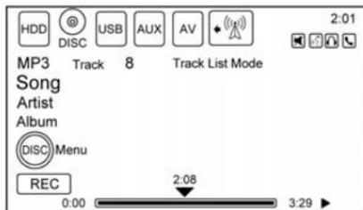
If a disc is already loaded, but you are currently on a map screen or listening to a different audio source, press SRCE to switch to the Disc source. A track number appears on the display when each track starts to play.
