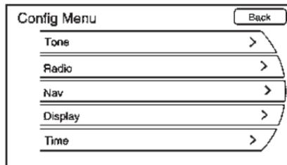
Press the Multifunction knob to enter the Config setup menu features. Turn the Multifunction knob until the Display feature displays. Press the Multifunction knob or press the Display screen button to display the other options.
