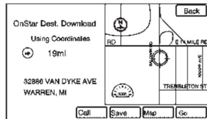
If the address is not found within the map database, the system may use latitude and longitude coordinates to locate the destination. In this case, “Using Coordinates” displays on the downloaded screen.
