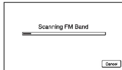
To find a list of local stations in the current AM or FM band, press the Multifunction knob or touch the audio source screen. The radio performs a search for available stations.
