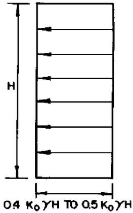
Where deformations are critical and tie-backs are prestressed to 100% of design load, compute pressure based on at-rest conditions. Use  $K_0 = 0.4$  for dense sand, and  $K_0 = 0.5$  for loose sand.
