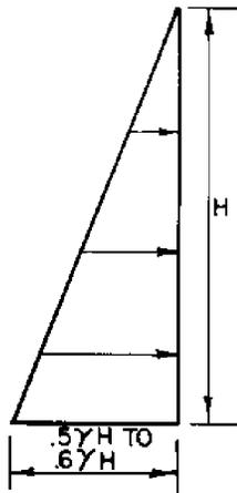
Compute pressure based on at-rest conditions with  $K_0$  from 0.5 to 0.6. In normally consolidated clays excessive prestressing should not be permitted because of the potential for induced consolidation. Use design procedure as in Figure 26.
