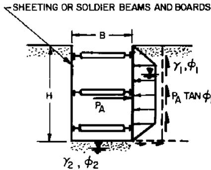
STABILITY IS INDEPENDENT OF H AND B, BUT VARIES WITH  $\gamma, \phi$  AND SEEPAGE CONDITION.
