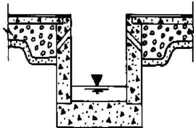
IF SOUND ROCK OR IMPERVIOUS STRATUM EXTENDING TO A GREAT DEPTH IS ENCOUNTERED AT SHALLOW DEPTH BELOW FOUNDATION, CARRY OUTSIDE WALL AS CUTOFF. DISPENSE WITH WALL DRAIN AND REPLACE CAP ON FLOOR SLAB WITH DAMPPROOFING. ARRANGE DISCHARGE FROM DRAINAGE SYSTEM TO PREVENT AERATION OF DRAINAGE COURSE.
