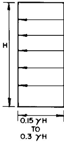
Use pressure ordinate to produce the same force as for braced excavation. 0.3 is applicable for stability number of about 4, and 0.15 is applicable when stability number is less than 4. Use design procedure as in Figure 26.
