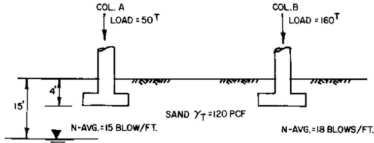
Column load A = 50 tons , Avg. N = 15 blows/ft.
