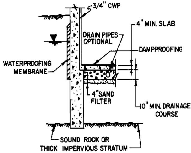
NOTE: IMPERVIOUS STRATUM OF SMALL THICKNESS MAY NOT BE ABLE TO WITHSTAND PRESSURE DUE TO HIGH WATER TABLE OUTSIDE THE FOUNDATION.
