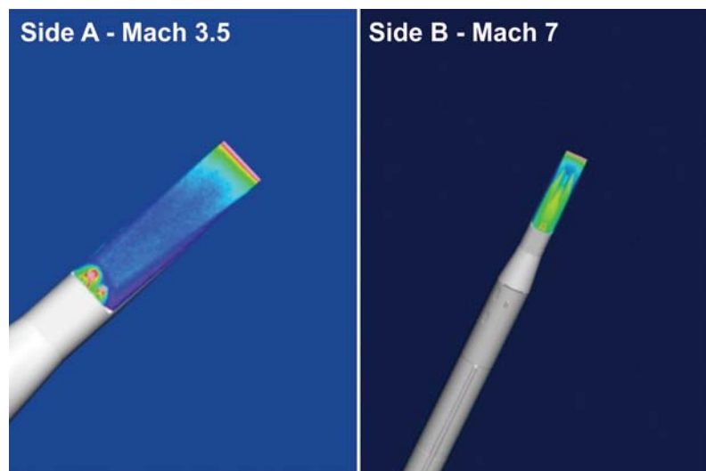
Figure 15: Optical simulation of the HyBoLT launch using an airborne system 5 miles from anticipated ground track.
