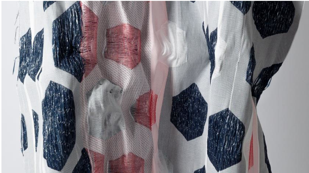
Figure 5: Kathryn Walters (2017). Introducing complexity and finding the limits of the loom. Attempted textile in polyester monofilament (transparent), elastic (red), and plastic tape yarn (blue). (c) Kathryn Walters.
