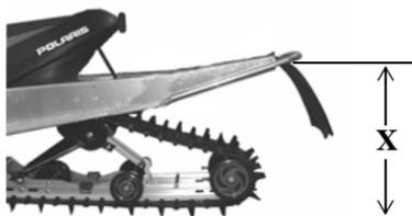
Take this measurement with no rider and with the rear suspension at full extension.
