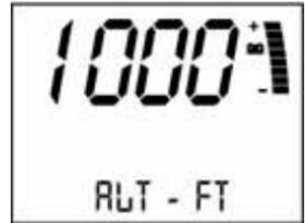
**TIP:** When "ALt-FT" displays, the program is in the standard mode. If only "Alt" displays, the program is in the metric mode.
