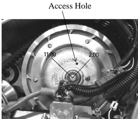
7. Locate the L-wrench in the tool kit. Install the wrench into the open threaded access hole in the outer sheave of the clutch.
