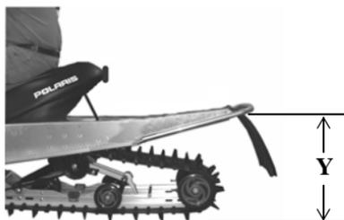
To determine sag, commonly referred to as ride-in, subtract measurement Y from X ( $\text{Sag} = X - Y$ ). Adjust sag by rotating the torsion spring preload cams located on the rear torque arm. See illustration. The ideal amount of sag for this rear suspension is five inches (12.7 cm) ( $X - Y = 5 \text{ in.} / 12.7 \text{ cm}$ ).
