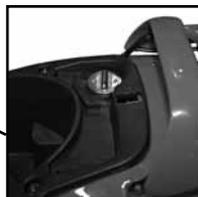
Locate gas cap under seat and remove, fill tank with new, clean 89 octane or higher gasoline. Do not overfill tank, do not fill over 1" below filler neck to allow for expansion. Gas tank capacity: 1.6 gal
