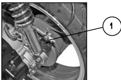
1. To make rear brake adjustment, turn rear adjusting nut (1) clockwise to increase and counterclockwise to reduce tension on the brake cable.
