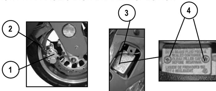
1. Inspect front disk brake caliper (1) for leakage. If brake fluid leaks, the safety of riding could be affected.
